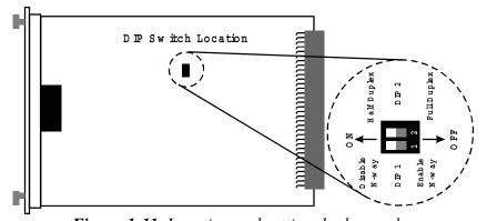
*Figure 1-11.* Location and setting duplex mode If you adjust to Enable N-Way, then the DIP for Half-Duplex and Full-Duplex is not effective. If you adjust to Disable N-Way, then the DIP for Half-Duplex and Full-Duplex is effective.
